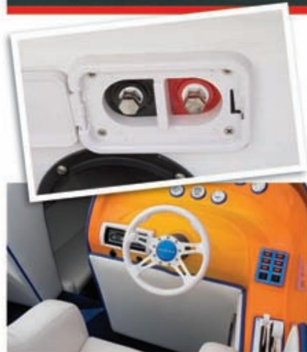
From above: B&H Performance included this remote battery access under the rear bench to charge the battery or provide a jump-start. The helm was completely color-coordinated.
